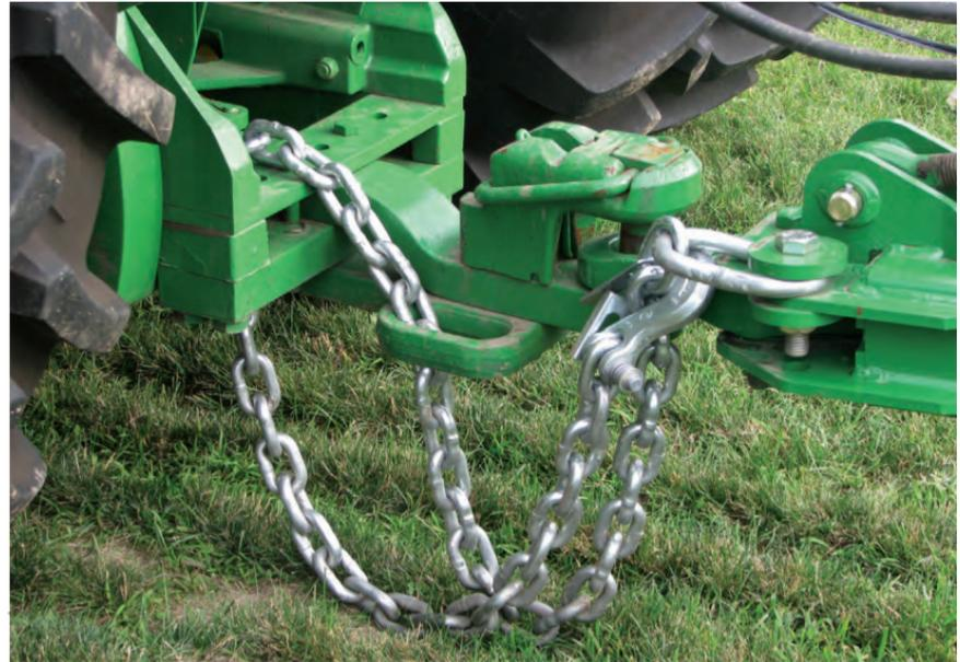
Safety chains a rate for a specific load. The load will be marked on a metal tag.
